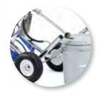
Inlet tube fits through a 2-inch cap opening on standard 5-gallon bucket.
